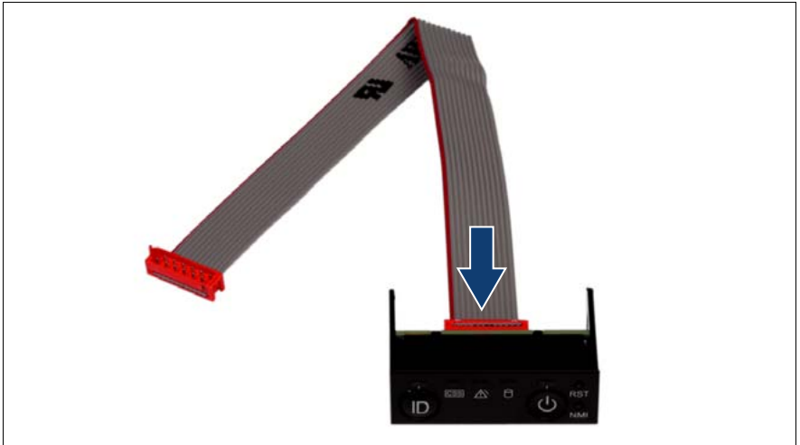
Figure 139: Connecting the control panel cable to the control panel
